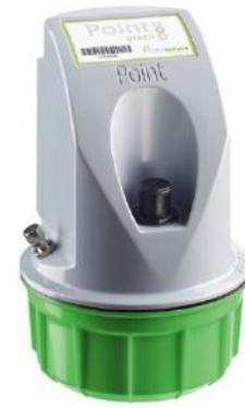
Point Green is a compact Logger/RTU device with integrated battery, a 3G modem with GPRS fallback, internal and/or external antenna, digital and counter inputs, Modbus and SDI-12 master capability and a submersion sensor.
